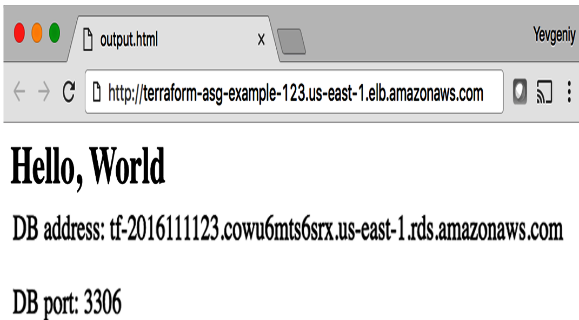
Figure 3-12. The web server cluster can programmatically access the database address and port.
